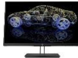
NEW! P/N: 1JS06A4 RRP €211 HP MONITOR Z23N 23" IPS, 1920x1080 FHD, 5MS, TILT, SWIVEL, PIVOT, HEIGHT ADJUSTABLE, 1 VGA, 1 HDMI, 1 DISPLAY PORT 1.2, 3 USB 3.0, 3YW
